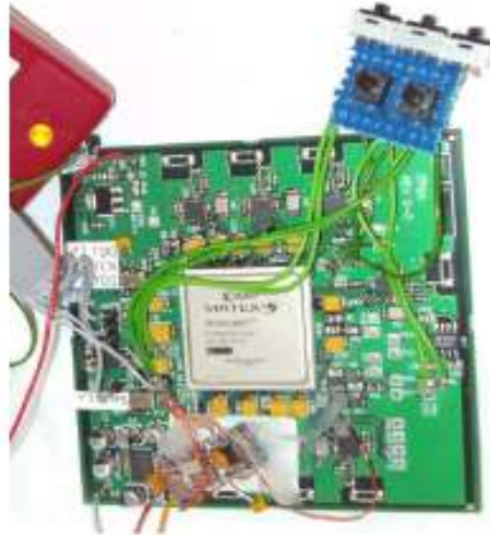
Figure 9: Node board for a custom FPGA (the "arms").
